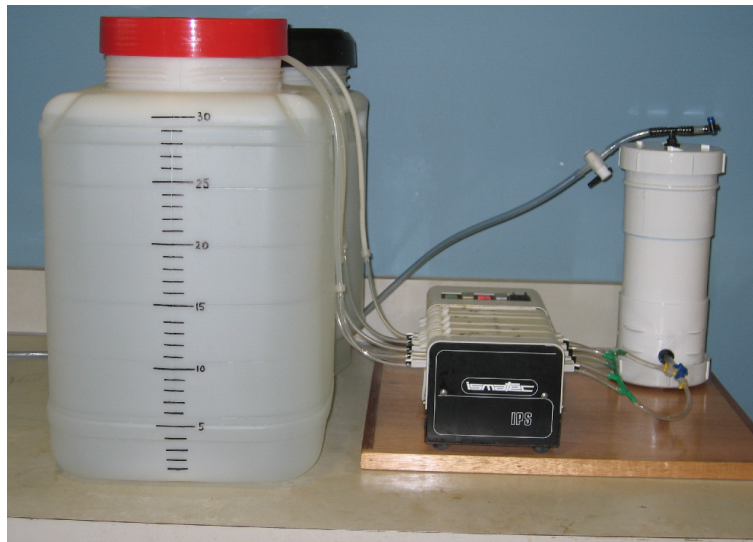
Above: Laboratory trial of activated alumina defluoridation column
