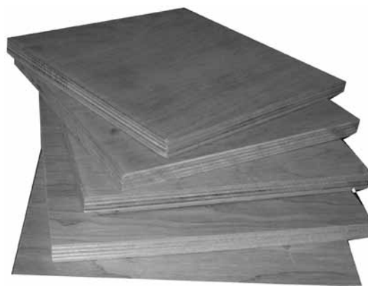
Top: A sheet of Plywood showing the face-side. Above: A stack of plywood showing the layers (plies) of wood glued together.
