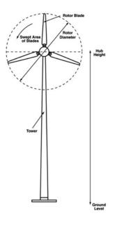
Maintenance of wind turbines can be a significant part of their lifecycle costs. The turbine must be lowered once a year, to service the generator, the blades and lubricate bearings. The generator will require a major overhaul every 4–5 years.
